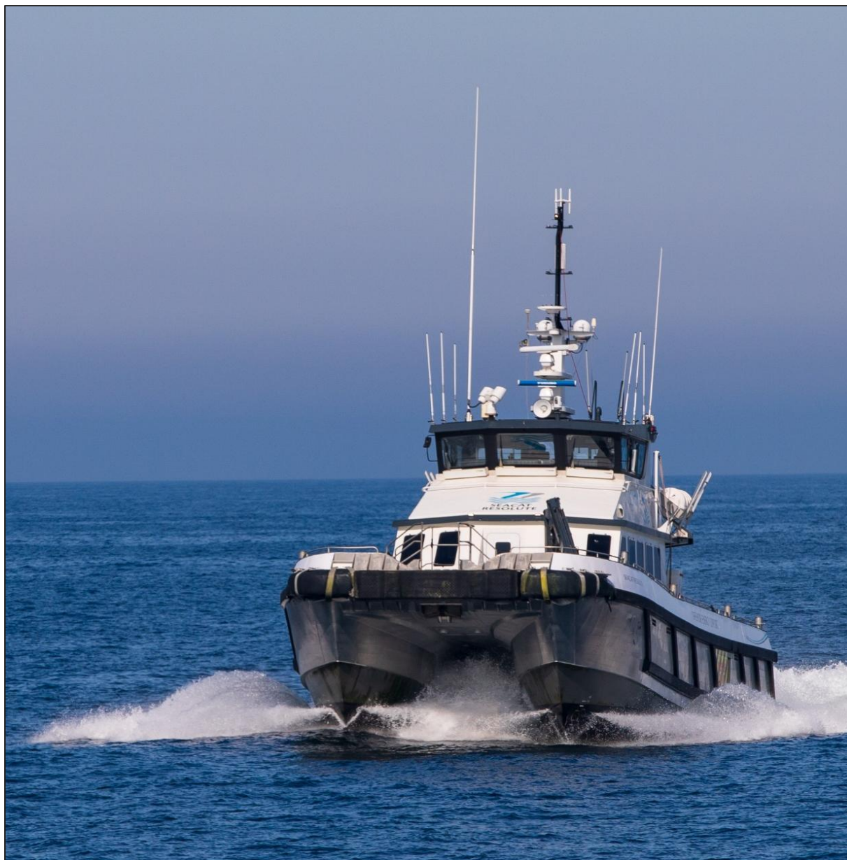
Figure 4.32: Crew Transfer vessel (Courtesy of Beatrice OWF)
