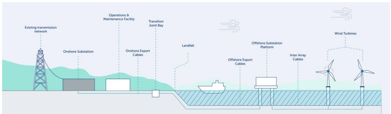
Figure 4.2: Main components of an offshore windfarm (OWF)
